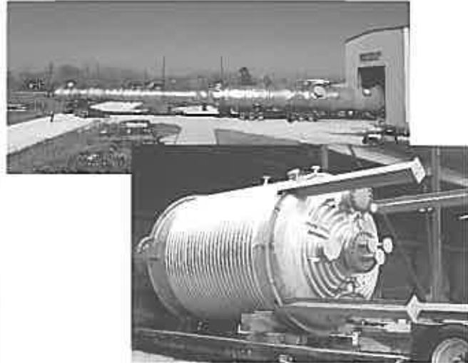
Vessels for cryogenic service, welded with DW-308L
