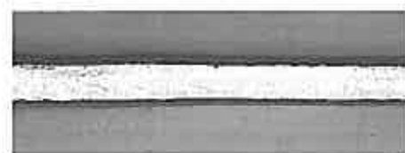
Fig.4 - The Glossy Bead Appearance of DW-308L
