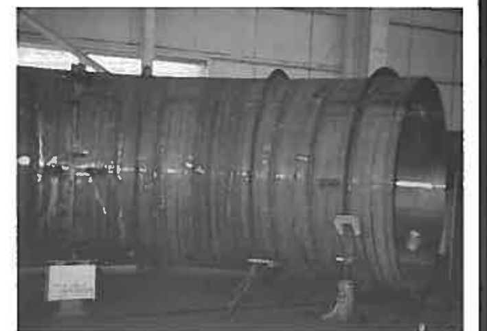
Fig.2 - A Water Pipe for the Water Gate Equipment under Fabrication by Using DW-308LP in All Positions
