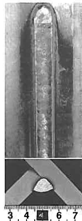
Figure 2. Bead appearance made in straight-run vertical-up fillet welding, having a smooth regular surface with no undercut
